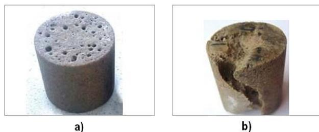
**Figure 1. Core samples after the modeling of hydrochloric acid treatment:**
